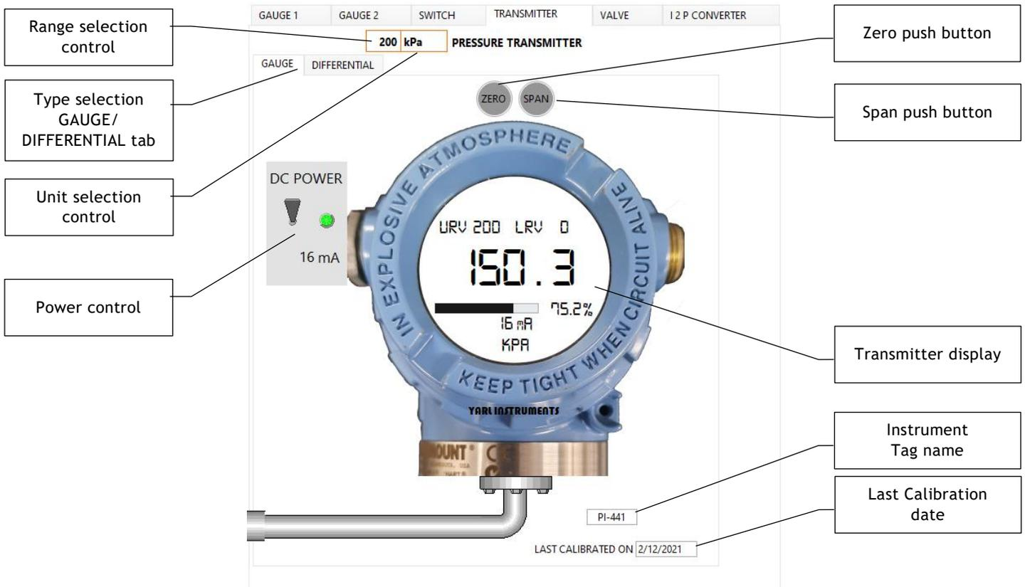
To calibrate a pressure gauge transmitter:
