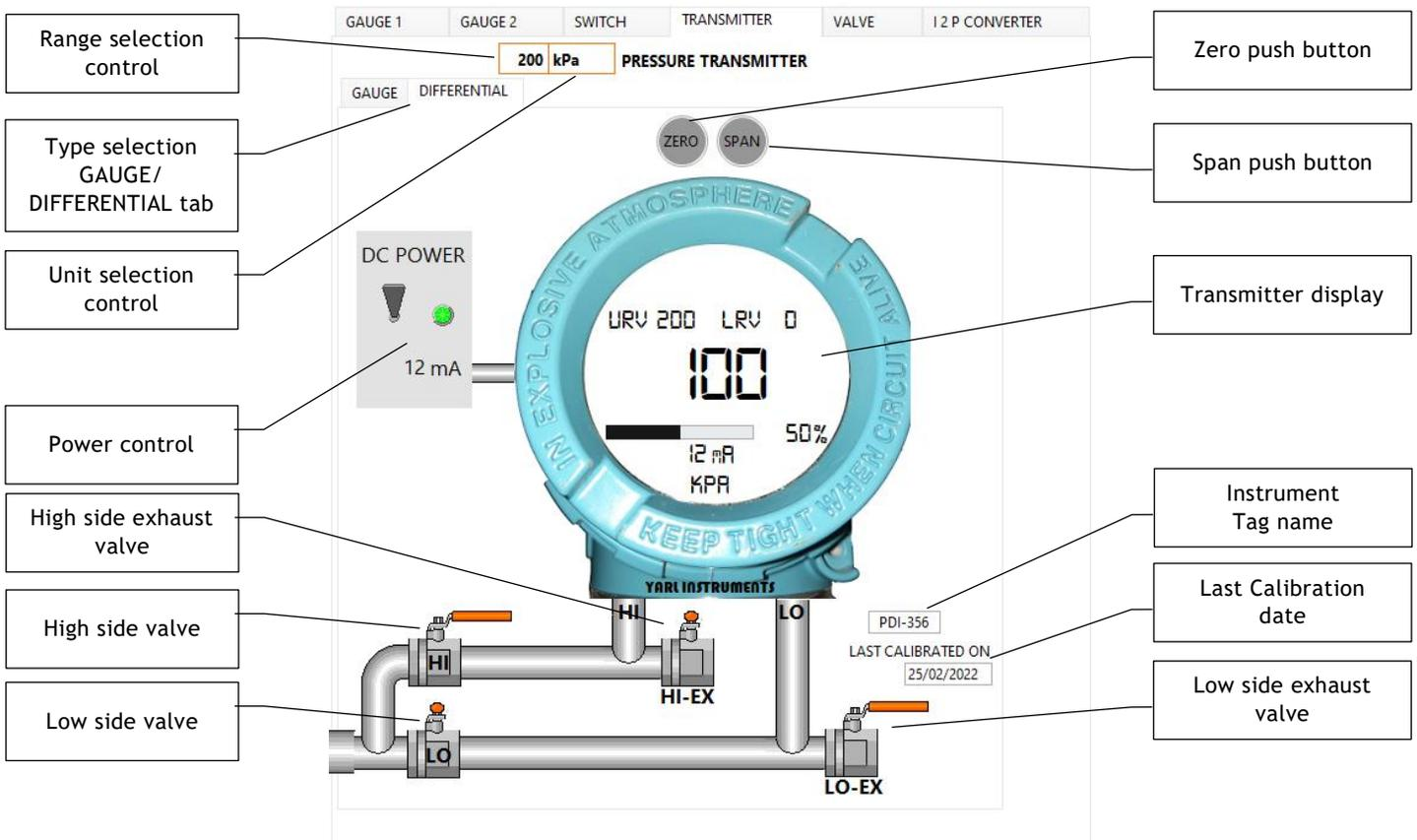
To calibrate a differential pressure gauge transmitter:
